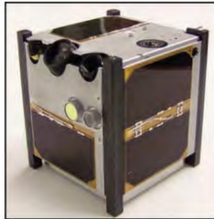
Aerospace Corporation CubeSat measures 10 by 10 by 10 centimeters, weighs 1 kg
