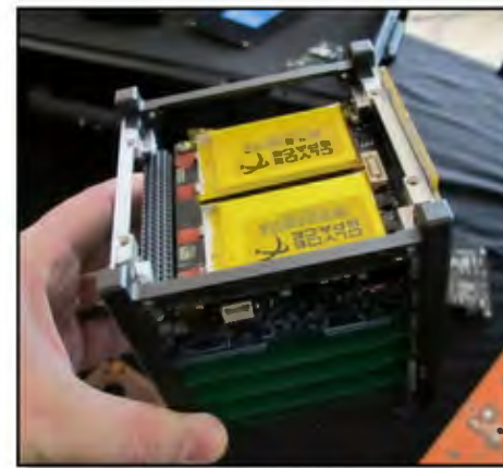
Aerospace Corporation CubeSat measures 10 by 10 by 10 centimeters, weighs 1 kg
